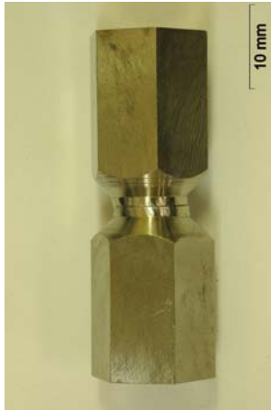
Classical thin wall tubular specimen
